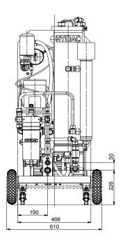
Dimensional tolerance ±10mm Dimensions in mm
